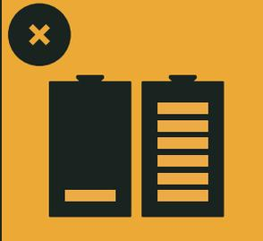
Batteries should be kept in the middle of their capacity. Draining the battery to 0% or charging over 80% reduces the battery-life.
