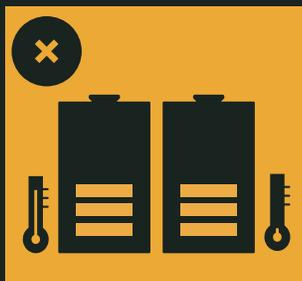
Store batteries and devices at room temperature and not in direct sunlight or below 32°F.
