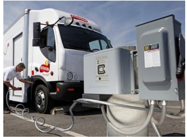
IMAGE 7. FRITO LAY COMMERCIALLY AVAILABLE TRUCKS SUCH AS SMITH ELECTRIC'S NEWTON, PICTURED ABOVE, USE THE STANDARD J1772 CONNECTOR, BUT MANY FLEETS USE PROPRIETARY ADAPTERS.
