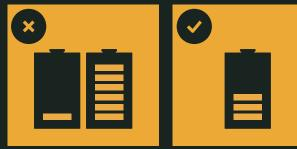
Batteries should be kept in the middle of their capacity. Draining the battery to 0% or charging over 80% reduces the battery-life.
