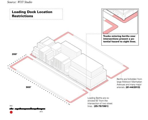
Figure 15. Loading dock location restriction as delineated in the zoning
